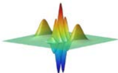
Figure: Theoretical Wigner Function of an Optical Schrödinger cat state, constituted by two coherent states clearly separated in the figure, and by oscillations in the center that are a signature of the quantum nature of the superposition.
