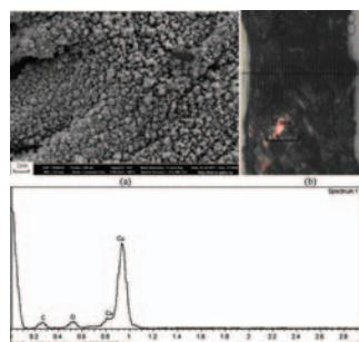
Image: SEM (a) and optical (b) microphotographs of the copper sediment made from the solution with sorbitol as reducer (the scale rate is given in the figure). (c) Presents the copper sediment EDX-spectrum.
