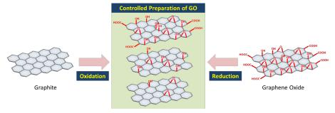
Applications such as conductive films, electrodes for lithium-ion batteries, super-capacitors and catalysts often require surface functionalization's to improve GO's performances. Recently, adsorbents and membranes for water purification have also been recognized as promising applications of graphene-like materials. With our tailor-made GO, we developed catalyst, membrane, lubricant additive and anode for Li-ion battery.
