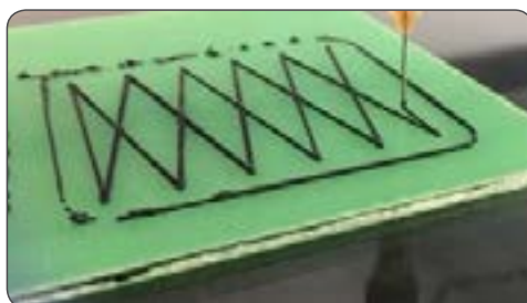
Fig. 1. Image of the 3D printed circuits based on nanoreinforced epoxy resin with carbon nanostructures
