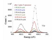
For example, thanks to quasi *in-situ* XPS, it will be shown why, after the surface passivation phase, more than 5 cycles PEALD are needed to restart growth of TiO, on Si, whereas growth starts at the first cycle on TiN
