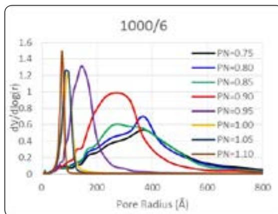
Figure 1: Pore size distribution of 70% ZrO<sub>2</sub> - 20% CeO<sub>2</sub> - 10% RE aged at 1000°C for 6 hrs as a function of the amount of complexing additive.
