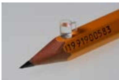
Figure 1: "The world's smallest beer mug" standing 5mm tall, fabricated by Selective Laser-Induced Etching
