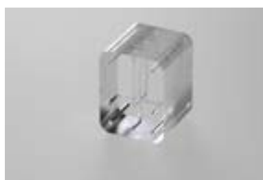
Figure 2: A novel glass microfluidic device for visualization of 3-dimensional elongational flows.
