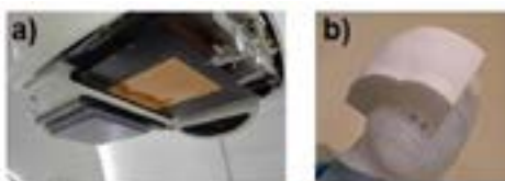
Figure 1. a) Range Shifter (RS) attached to the beam nozzle and b) printed compensator, attached to the patient's mask.
