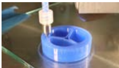
Figure 1: One example of 3D printed silicone object designed for printing valves
