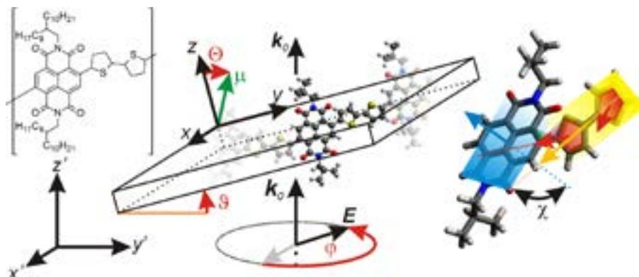
Schematic of the IR TMOA measurement geometry. [2] The combination of inclination( $\Theta$ )- and polarization( $\varphi$ )-dependent analysis enables to determine the orientation of atomistic planes relative to the substrate ( $\Theta$ ), and hence, relative to each other ( $\chi$ ).
